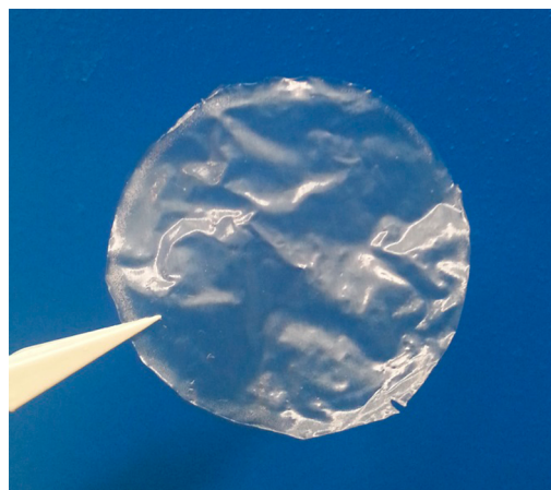
Figure 7. Standalone PEC film (1 inch diameter and 15 \mu\text{m} thickness) spun from PSS/PDADMA coacervate in 1.7 M KBr at 1000 rpm.
